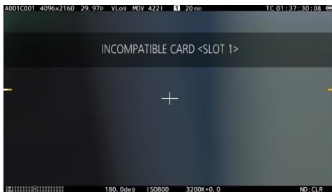
Fig.1 Message displayed when mounting an SD card of a lower video speed class than required for the codec selected on the camera.
